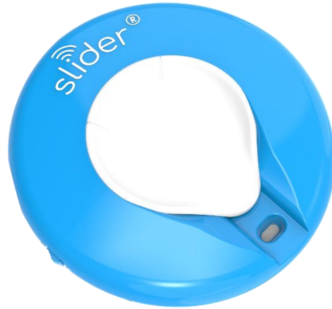
Figure 1 The Slider device- a pressure sensor and optical tracker which fit under the heel during self-directed physiotherapy sessions
