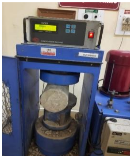
Figure 3 Test set up and cylinder specimen detail for tensile strength
