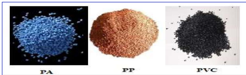
Figure 2 : Appearance of the granules of PA (a), PP (b) and PVC(c) ) belonging to the particle size class 2 to 4 mm
