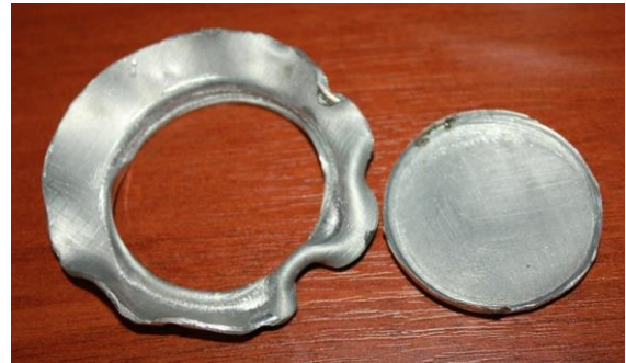
Fig. 5. Pulling down of the workpiece part and its destruction in the form of the separation of the bottom.
