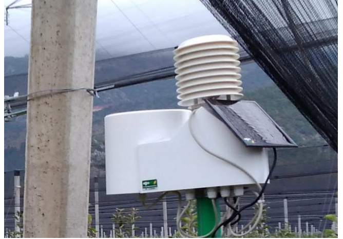
Figure 4. Sensor node for measuring air quality parameters.
