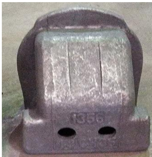
Fig.3. FWVD from synthetic cast iron in a one-time sand form
